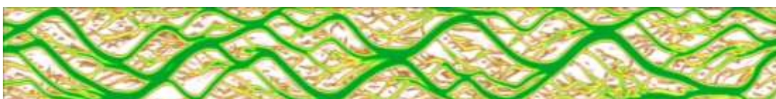
Fig.1 Numerical simulation of the development of a braided river using iSWEM
